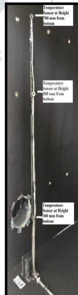
Figure 7. Temperature measuring fixture
